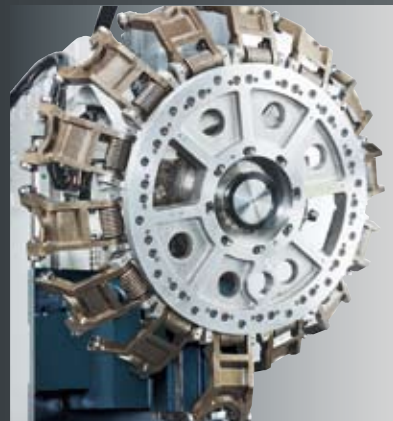
Armless-Type Magazine Tool change time: 1.8 sec. 12 and 14 tools are available
